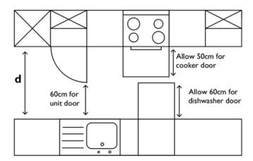
Most unit doors open up to a maximum of 60 cm. Dishwashers doors usually open by 60 cm and oven doors usually about 50 cm.
